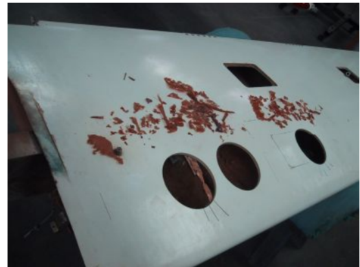
Figure 1. Loose Epoxy Flakes
