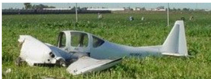
Figure 3. Broken Left Wing,
