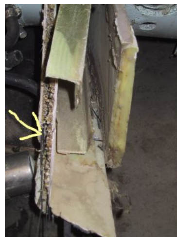
Figure 4. View of broken main spar box
